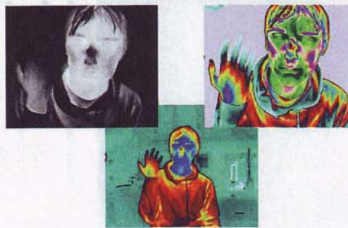
Pictures taken with a Type-II superlattice infrared camera detecting light between 3 and 5 \mu\text{m} .
